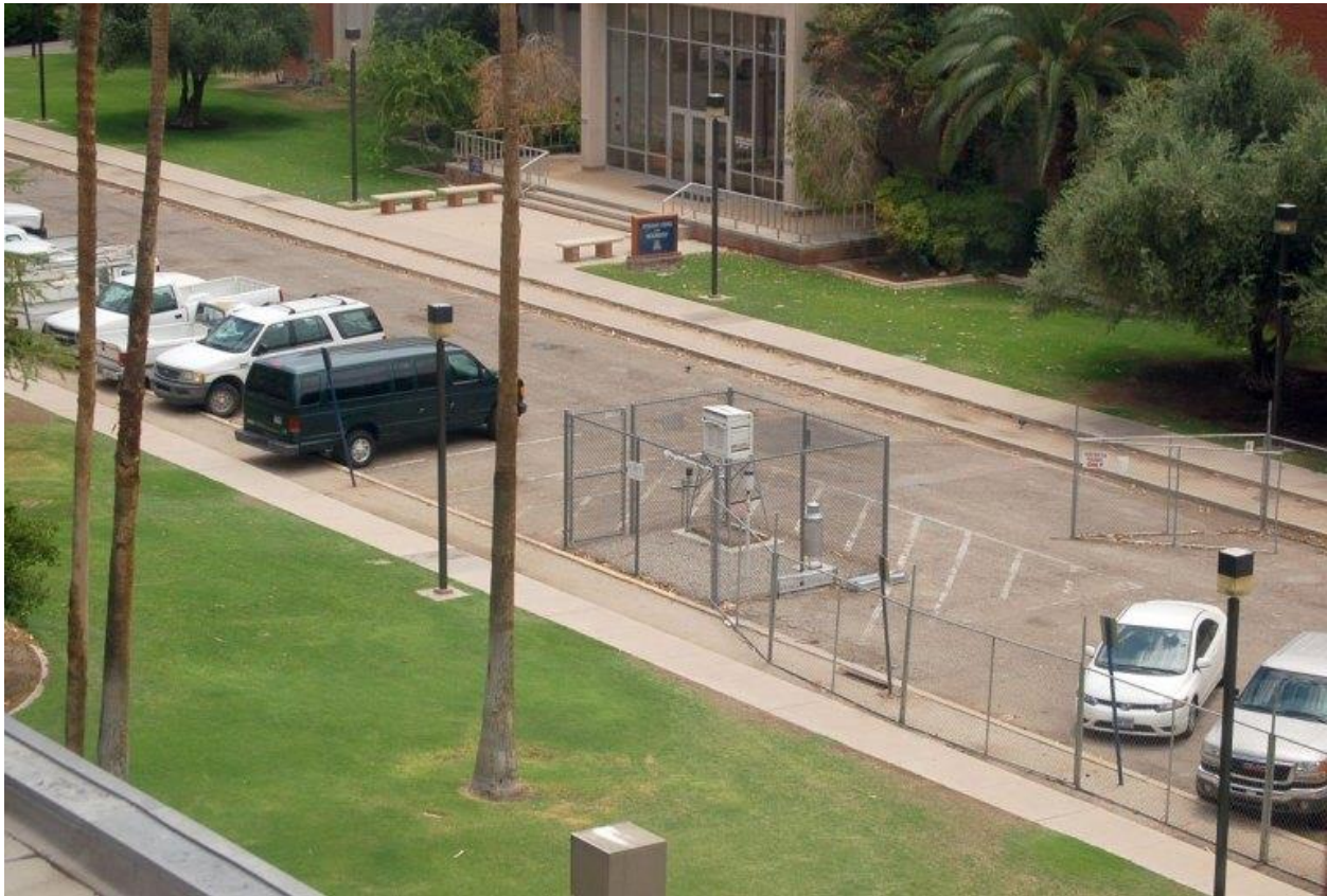
Figure 1 - USHCN weather station used for climate data in a parking lot. University of Arizona Atmospheric Sciences Department, Tucson. The station had previously been in a grassy area but was moved as the campus grew.
